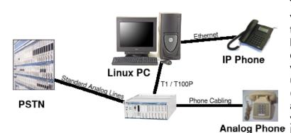
This diagram shows another variation on the Asterisk PBX theme. Here, 8 incoming phone lines, and 16 outgoing stations are connected to a channel bank, which is connected to Asterisk using a T1 cross over cable (remember, in this diagram T1 is just a technology, not a service that you have to pay for). A T100P from LSS then performs all the PBX functionality, using the channel
